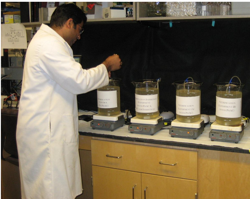
Figure V-2: Batch bioreactor experimental setup Mixed liquor from the SBR was used as biomass seed in the batch experiments
