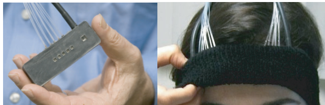
Figure 2: (Left) An fNIRS probe with four light sources and one detector. (Right) A researcher secures two fNIRS probes on a volunteer’s forehead. This arrangement is used to measure the prefrontal cortex (PFC)
