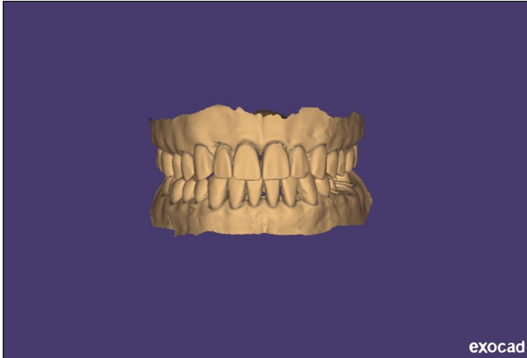
Figure 21: The STL file before exporting as one object with the recorded relationship.
