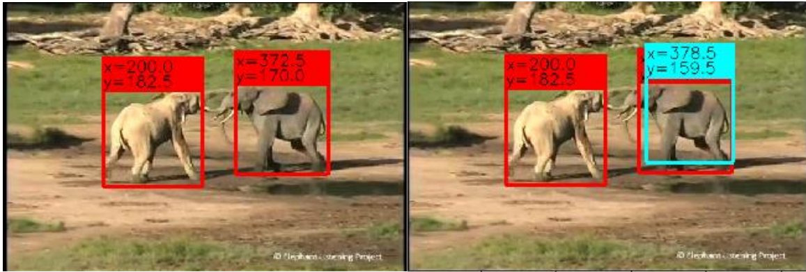
Figure 4-17: Elephant tracking results of the Kalman-filter-based tracker. The frames shown in this figure are extracted from a video sequence at multiple time stamps. The red bounding boxes are the ground-truth bounding boxes, while the light-blue boxes represent the predicted bounding boxes for the respective objects of interest.
