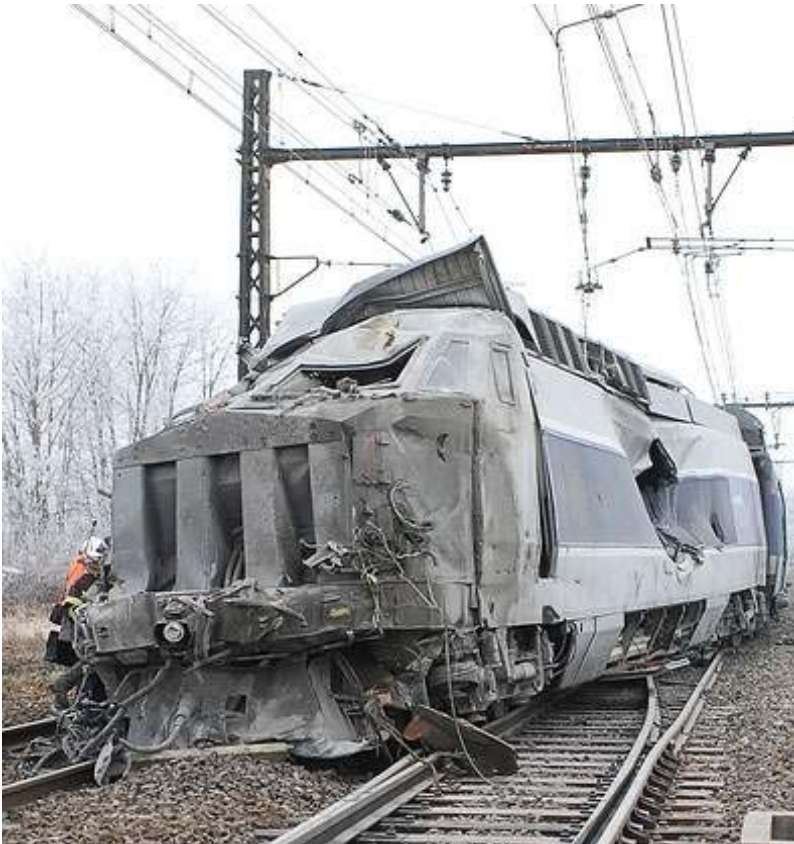
Figure 56: Damage to the Powercar at Tossiat
