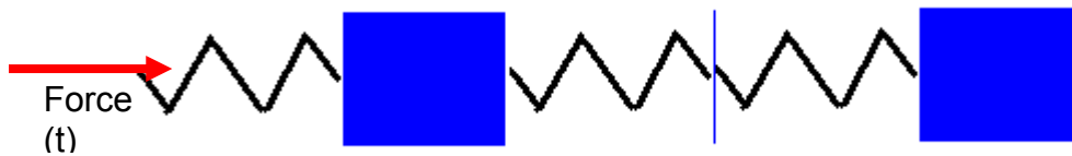
Figure 32: Force Applied to an Expanded Spring-Mass System
