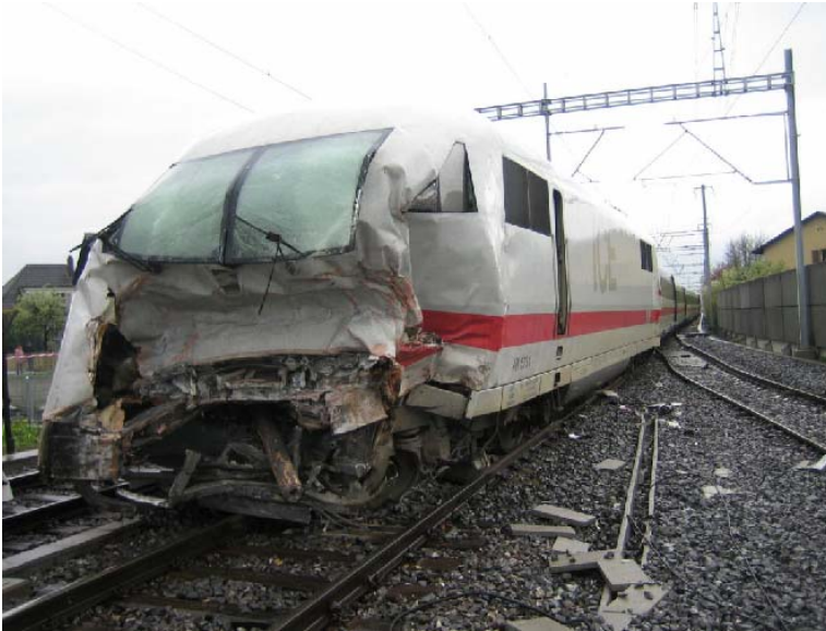
Figure 55: Damage to the Powercar at Thun
