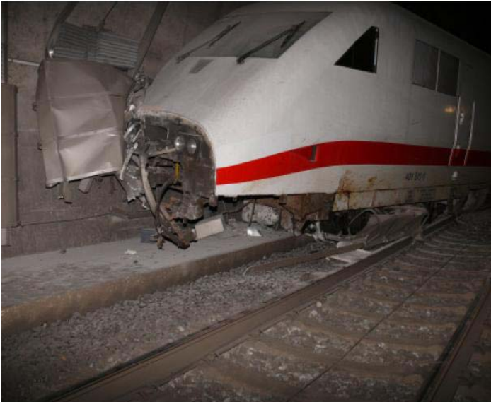
Figure 57: Damage to the Powercar at Fulda
