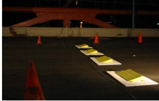
Fig. 7. Steel ramps used in the tests
