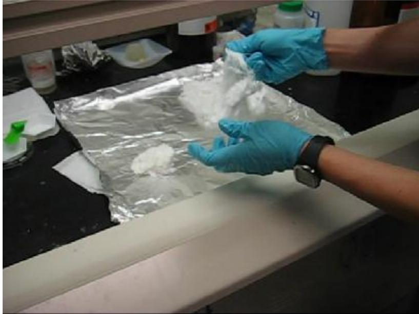
Figure 3. Silk laid out in fume hood to dry.
