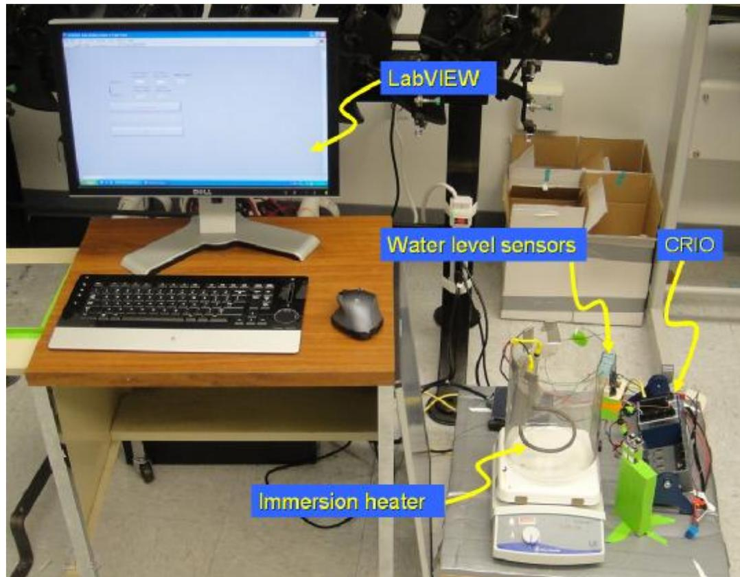
Figure 7. Silk automated boiling system.
