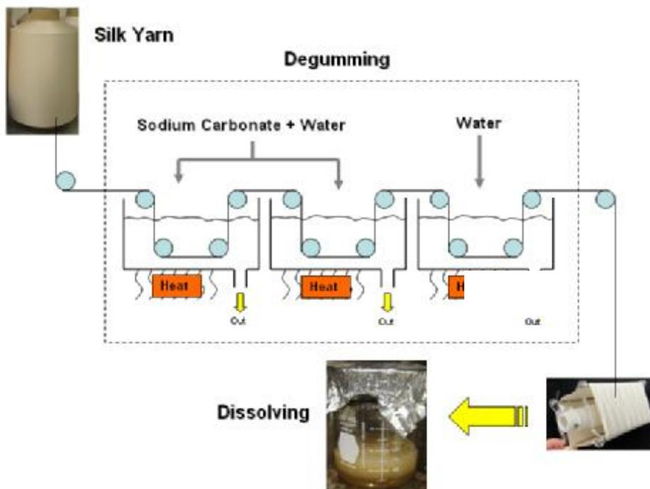
Figure 26. Bave silk yarn continuous degumming
