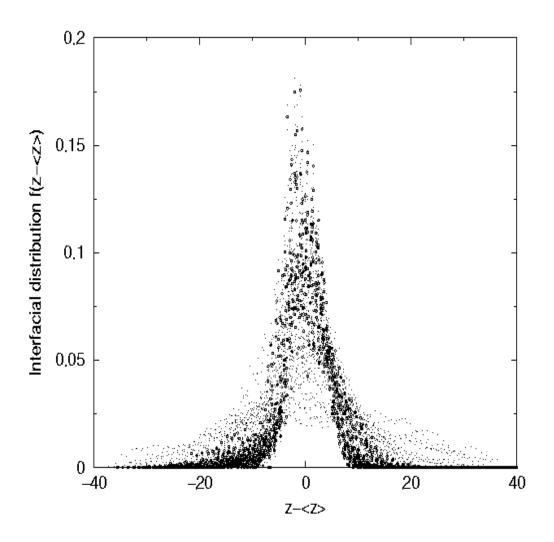
Figure 11: Scaled interfacial distributions for binary invasion (squares) and invasive water: surfact ant ratio 2:1 (points).
