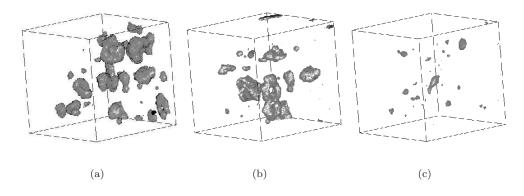
Figure 9: Isosurface of residual oil at timestep 20000. a) No surfactant. b) Water-surfactant ratio 4 : 1. c) Water-surfactant ratio 2 : 1. Isosurface shows oil concentration at a value of 5 particles per site. Forcing level 0.01. Porous media is not displayed for clarity.
