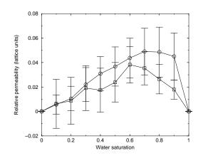
Figure 3: Variation of the off-diagonal components of the relative permeability matrix  $k_{ij}$  with wetting fluid saturation. The squares show relative permeability for oil (non-wetting fluid) when water is forced, the circles show relative permeability for water (wetting fluid) when oil is forced.
