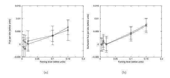
Figure 5: Fluid-fluid coupling for steady state ternary amphiphilic flow. System size  $64^3$ . a) Oil flux (squares) and water flux (circles) when water and oil are forced, respectively. Fluxes measured for a water saturation of 0.7. b) Surfactant flux when oil is forced (squares), and when water is forced (circles).
