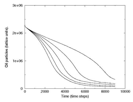
Figure 6: Number of oil particles in system as a function of time for various forcing levels in a binary system. The forcing level is from right to left 0.01, 0.02, 0.03, 0.04, 0.05 (lattice units). Error bars show the standard deviation on the mean of five independent simulations.
