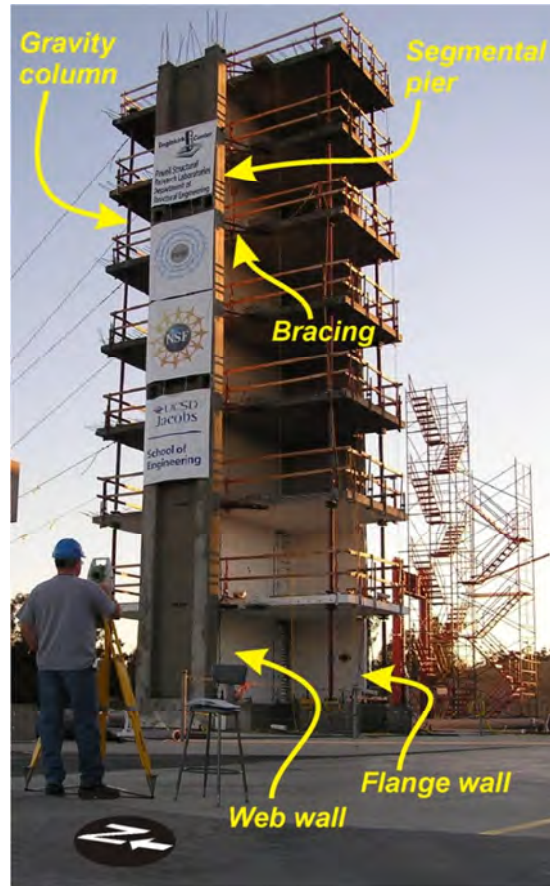
Figure 13. Full-scale shear wall test structure
