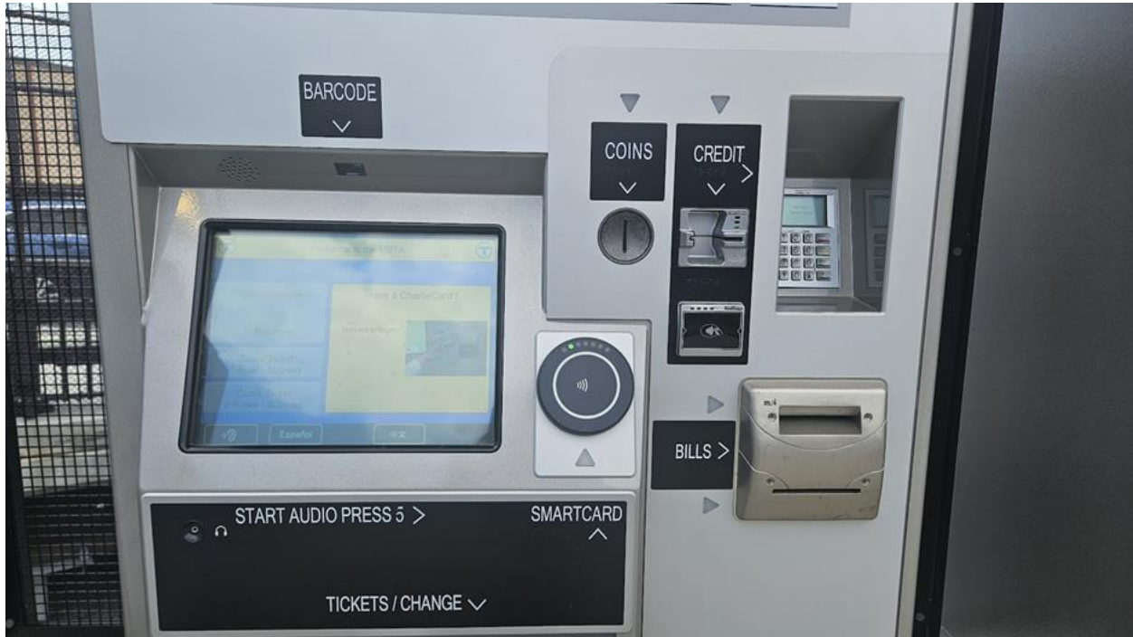
Figure 8.1: Tactile-Braille signage at an MBTA fare kiosk
