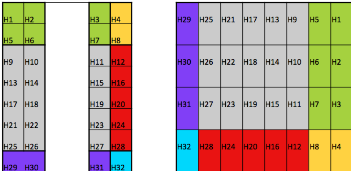
Figure 16: The mapping of heater switches to the module surface. The left diagram represents the heater switches and the right diagram represents the corresponding heater locations looking down at the module face.
