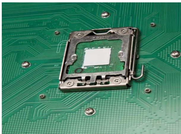
Figure 18: The latching mechanism clamps down around the edges of the module creating an electrical path between the module and the PCB
