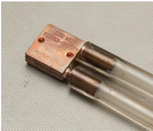
Figure 19: The liquid cooled heat sink used on the thermal test stand
