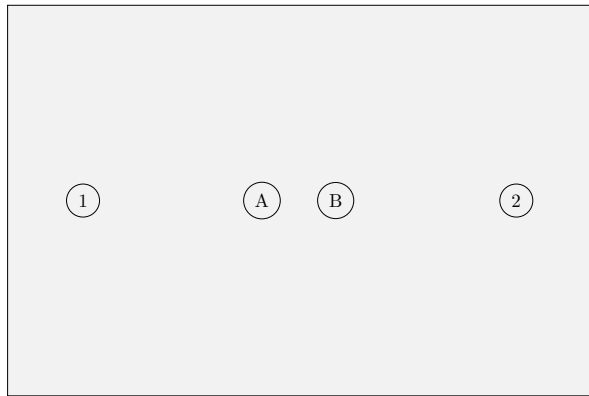
(a) fNIRS probe geometry configured for the dual-slope method [44]. It has 2 source locations and 2 detector locations (A and B). Each source location contains two light sources, one at 830nm and the other 690nm. Long source-detector distances (1-B, 2-A) are 35mm from each detector, and short source-detector distances (1-A, 2-B) are 25mm.
