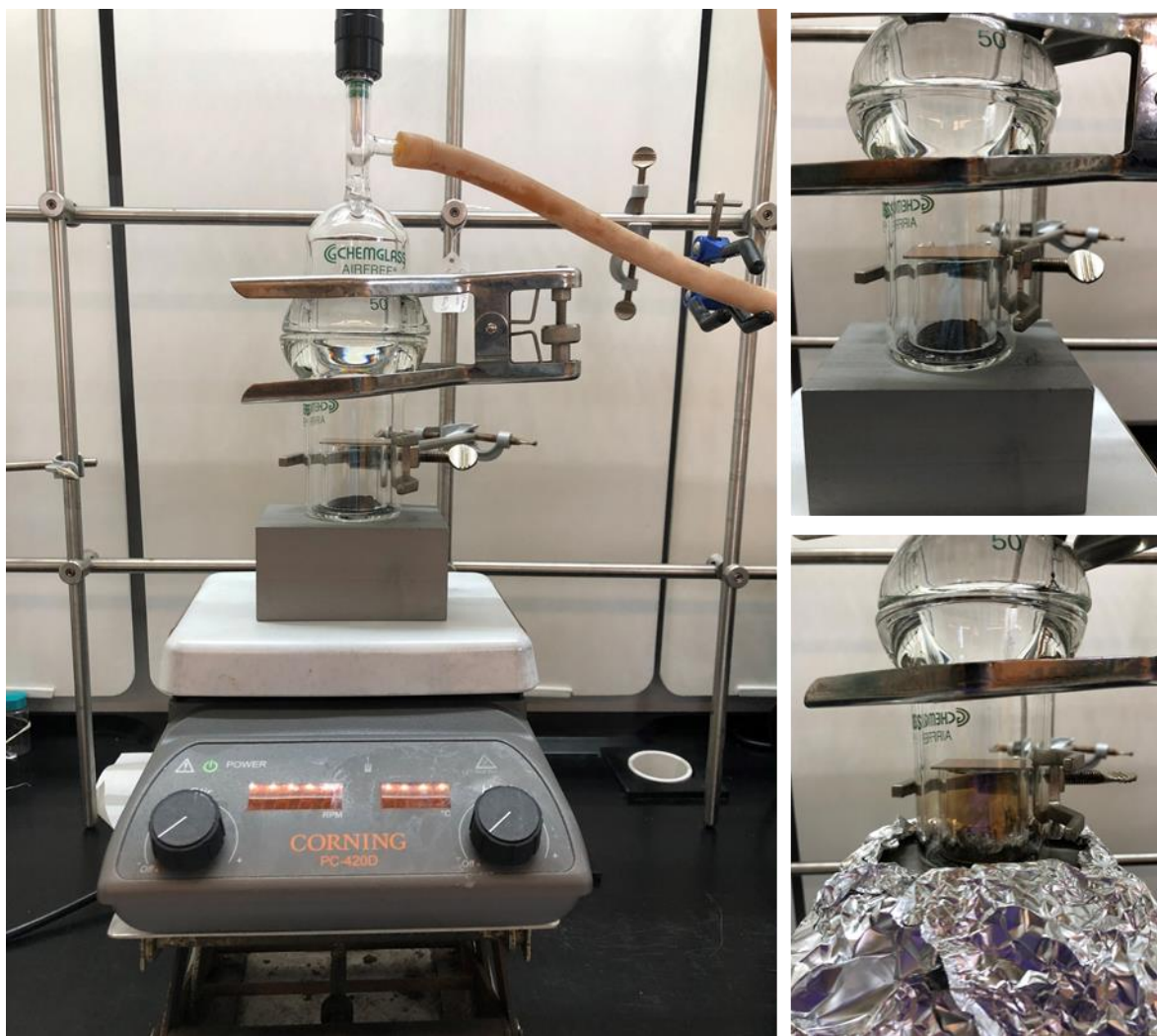
Figure 4.1. Photographs of deposition chamber set-up: (a) 50-mm Schlenk drying chamber on Al block on hot plate; (b) close-up of deposition chamber showing an inverted substrate supported by a 3.5-cm glass ring, with GeS powder loaded inside the glass ring; (c) Al foil wrapped around the block during a GeS film deposition—the GeS vapor can be seen as a brown gas.
