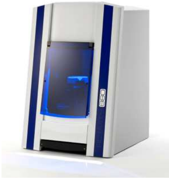
Figure 6. The Desktop scanner (Activity 880 scanner; Smart Optics, Bochum, Germany) used to digitize all the casts.
