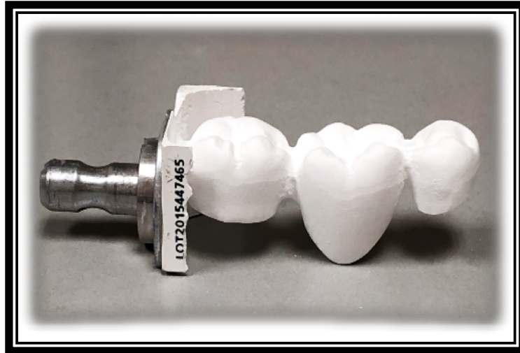
Figure 12: Milled Block of TZI Incoris Zirconia
