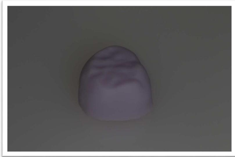
*Figure 5: Crown after milling and detaching from the block stump.*
