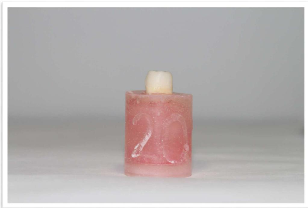
*Figure 9: Sample number 20 after being cured and cleaned of excess cement.*
