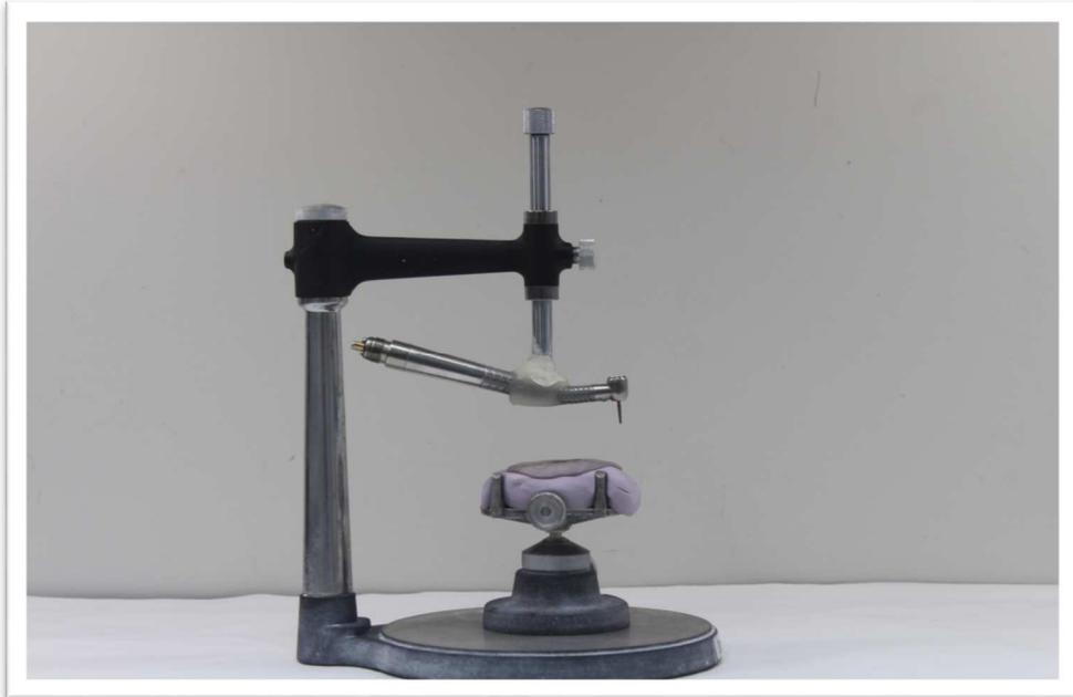
*Figure 1: Secured handpiece on a surveyor and the custom putty jig.*
