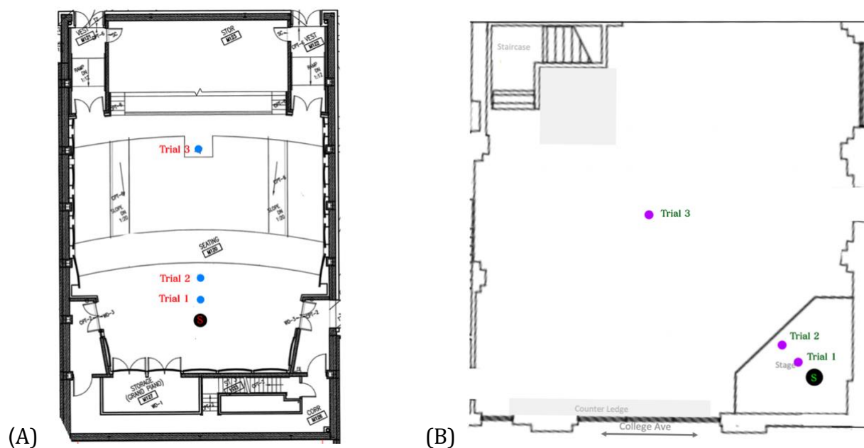
Figure 1. Layouts of Distler Hall and Curtis Multipurpose room. Black circle with S are source position. Colored dots are the relative positions of the receivers for each set of trials.
