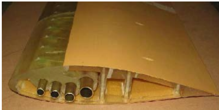
Figure 2-6: Wind tunnel model of NACA 63-421 with internal features for AJVG
