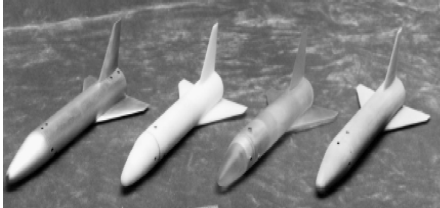
Figure 2-7: Wing-body wind tunnel models (left to right), aluminum, FDM-ABS, SLA, and SLS [15]
