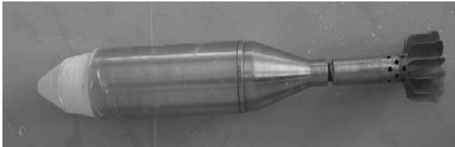
Figure 2-10: Steel model of missile with 3DP nose [31]
