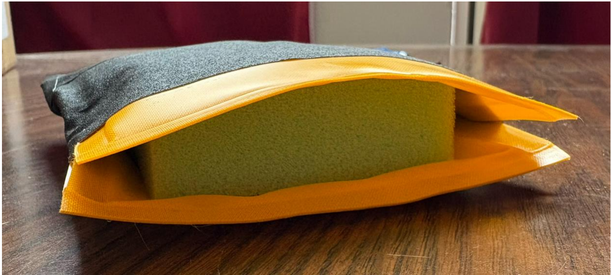
Figure 4. Internal cross section view of interface revealing viscoelastic core.
