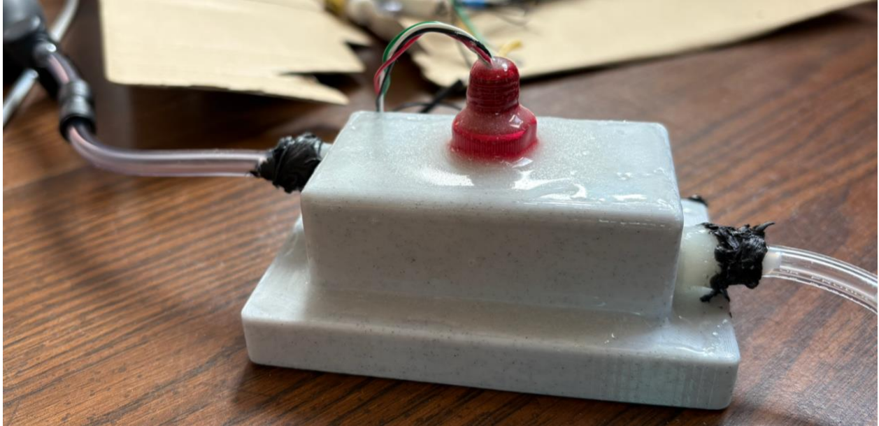
Figure 3. Reservoir with mounted barometric pressure sensor for interface inflation calibration.
