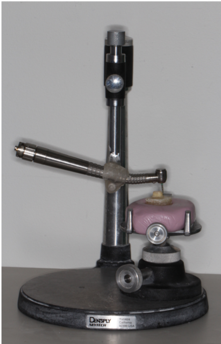
(Figure 3.B): A custom jig on the surveyor table held immovably in the surveyor base
