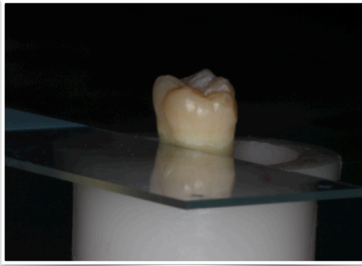
(Figure 1.B): A sample fixed vertically inside the mounting template with the CEJ being 1.0 mm higher than the top of a mounting template.
