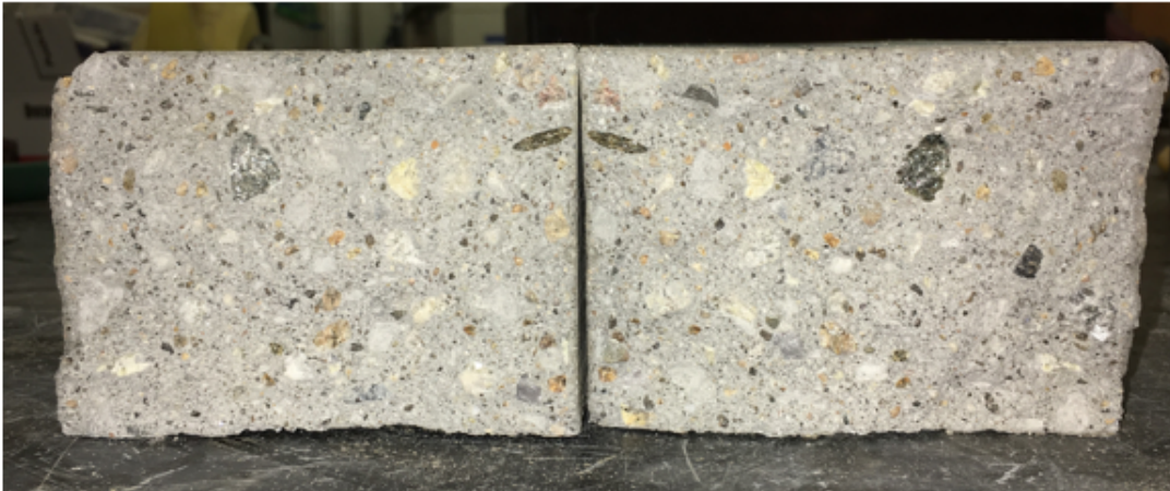
Figure 35 - Specimen #1 failure cross-section
