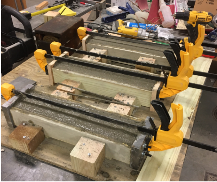
Figure 12 - Freshly poured concrete in specimen molds
