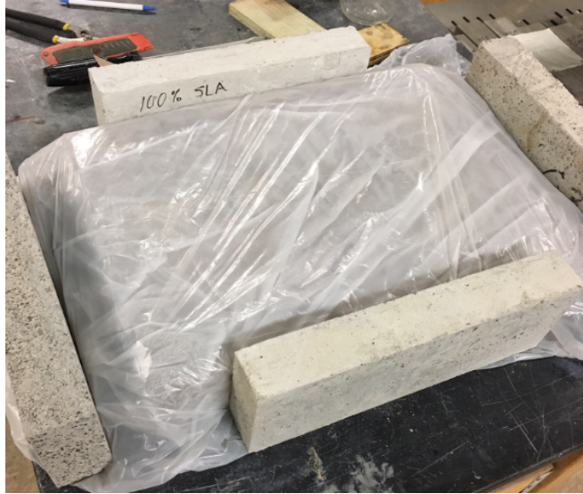
Figure 15 - Plastic seal over curing specimens
