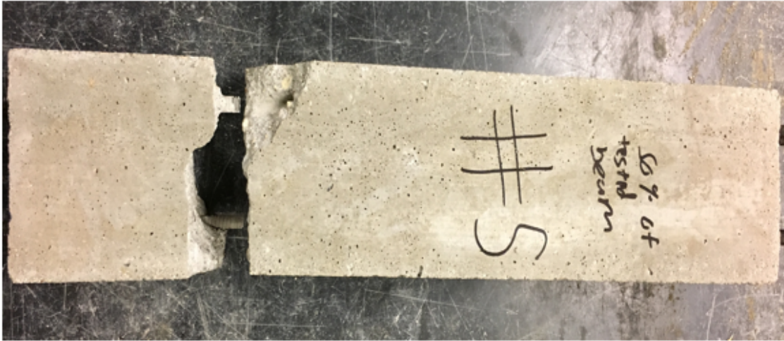
Figure 42 - Specimen #5 failure plan view
