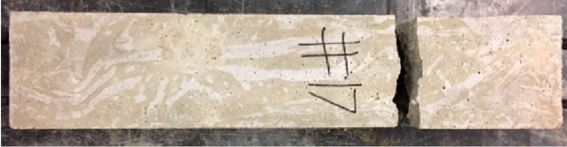
Figure 69 - Specimen #17 failure plan view
