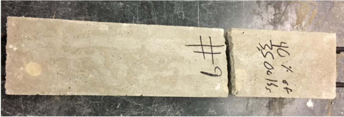
Figure 51 - Specimen #9 failure plan view
