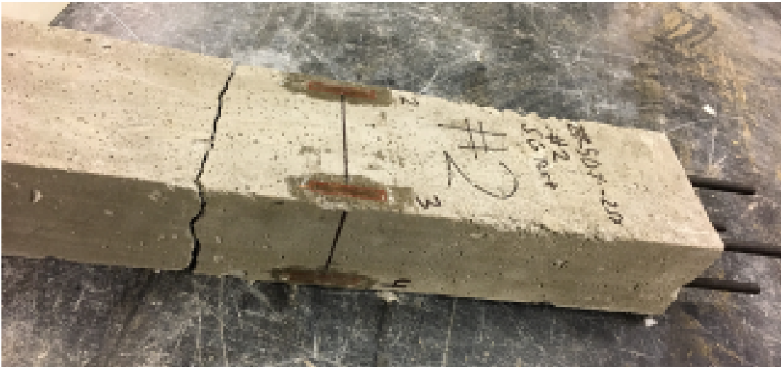
Figure 31 - #2, 3, 4 strain gauge layout
