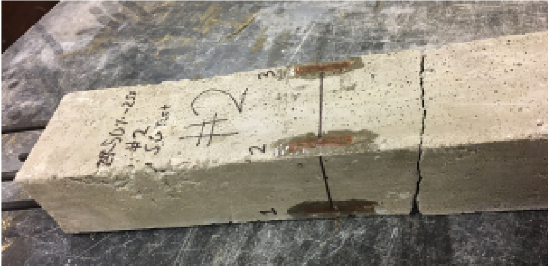
Figure 30 - # 1, 2, 3 strain gauge layout
