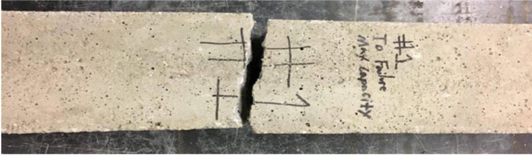
Figure 34 - Specimen #1 failure plane view
