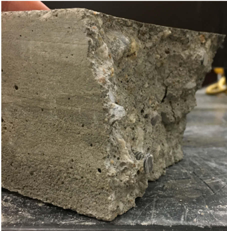
Figure 21 - Failure plane between the two longer rebar
