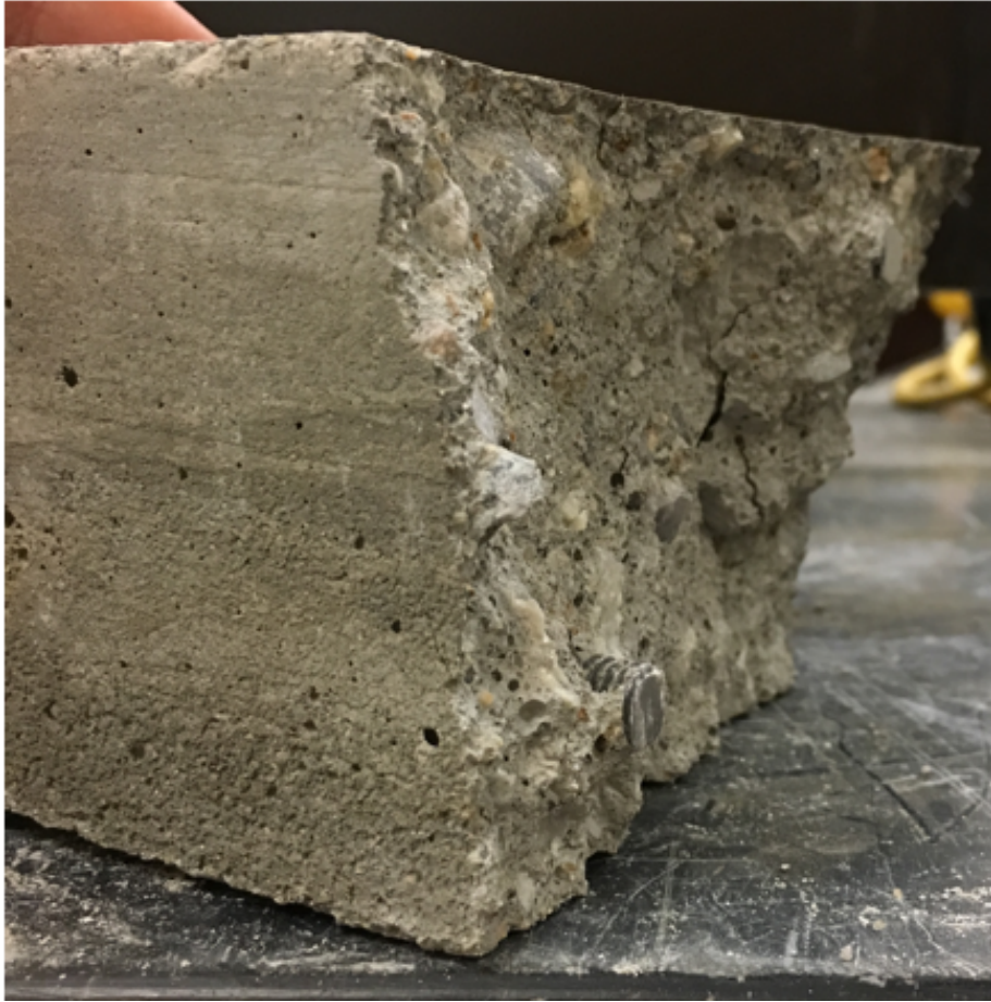
Figure 60 - Specimen #12 failure path
