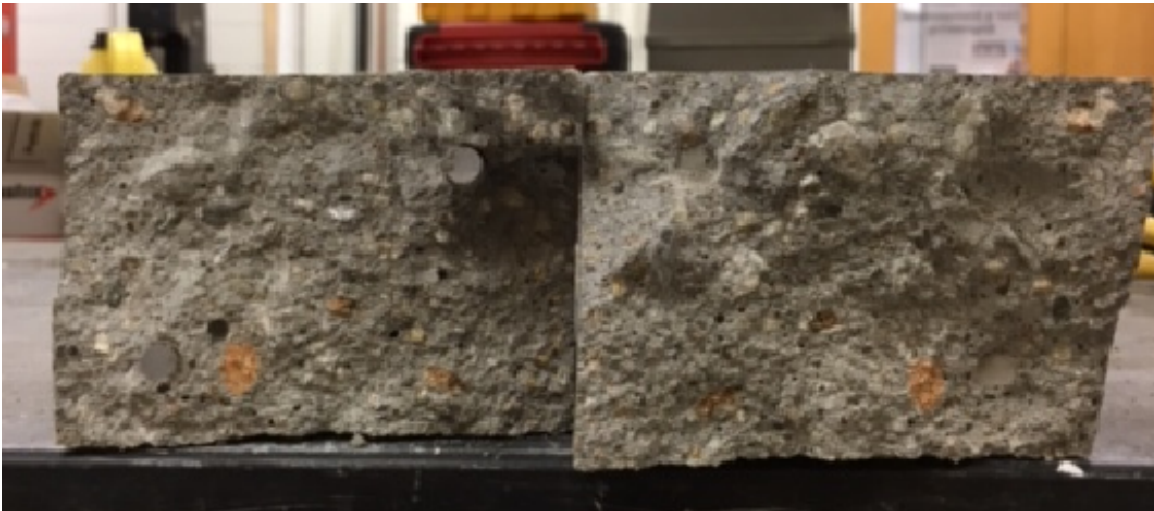
Figure 68 - Specimen #16 failure cross-section
