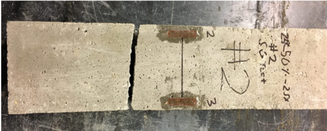
Figure 36 - Specimen #2 failure plan view
