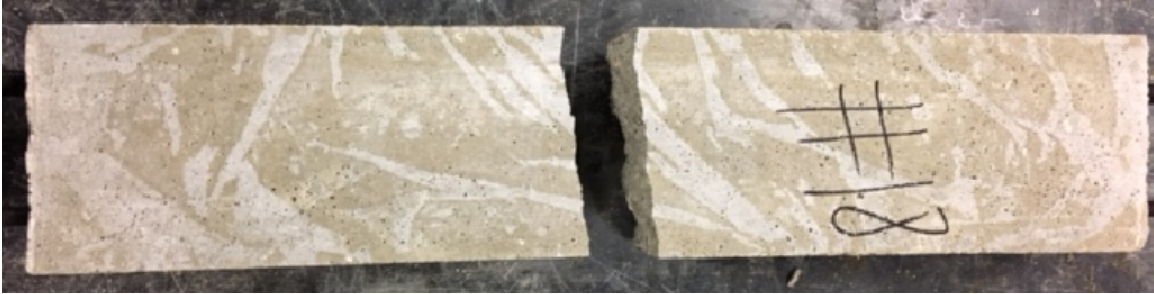
Figure 71 - Specimen #18 failure plan view
