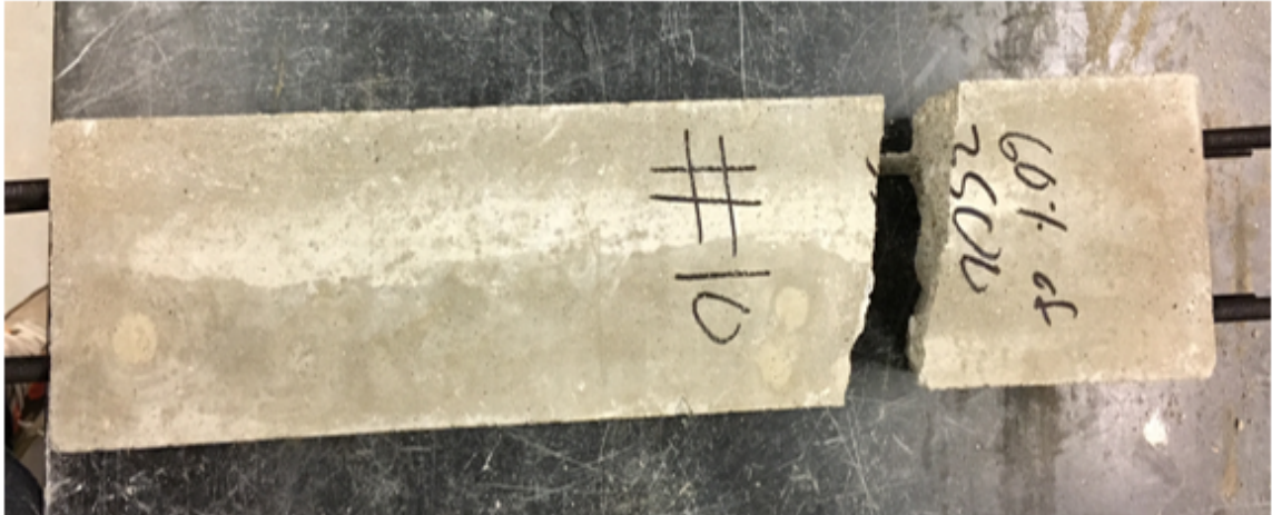
Figure 53 - Specimen #10 failure plan view
