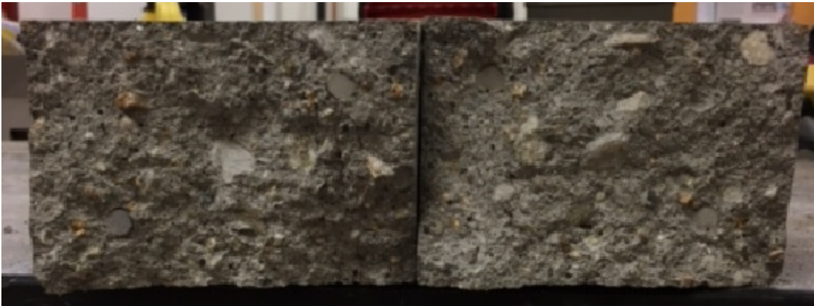
Figure 70 - Specimen #17 failure cross-section
