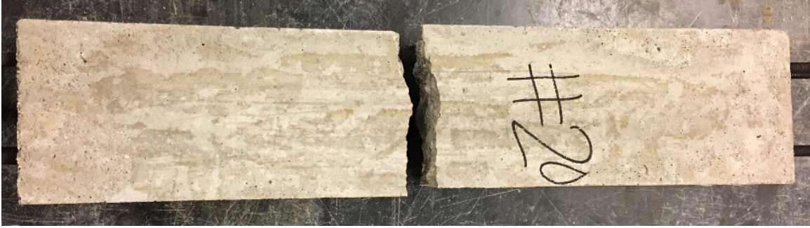
Figure 75 - Specimen #20 failure plan view
