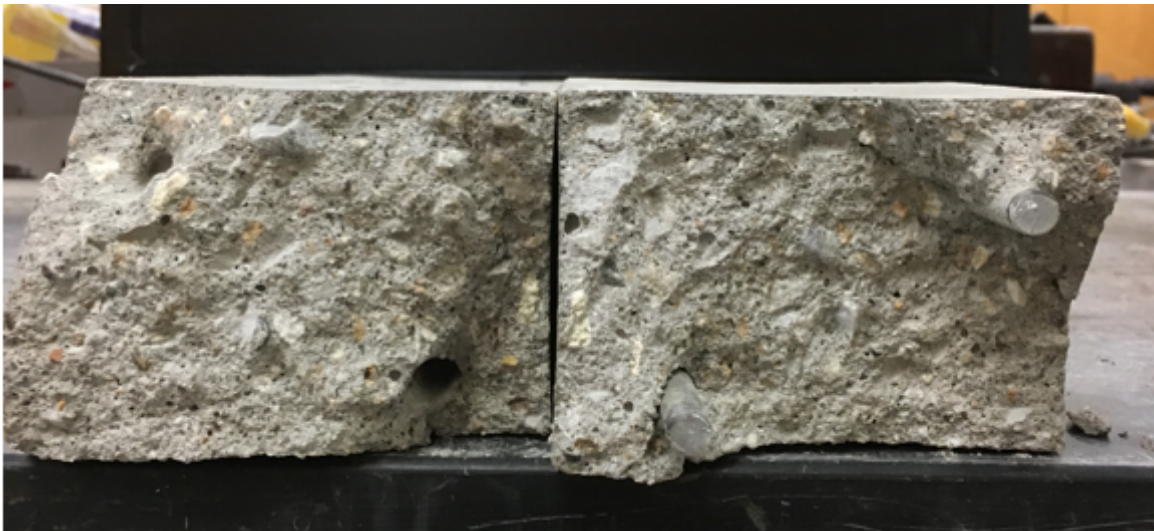
Figure 43 - Specimen #5 failure cross-section
