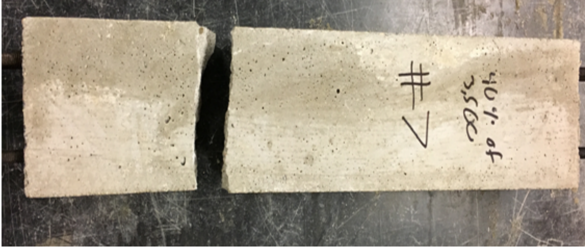
Figure 47 - Specimen #7 failure plan view
