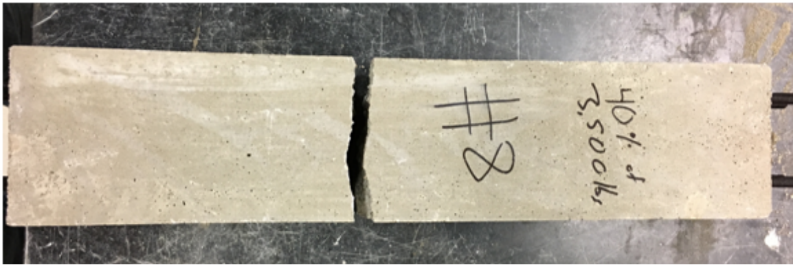
Figure 18 – Failure plane in unreinforced section
