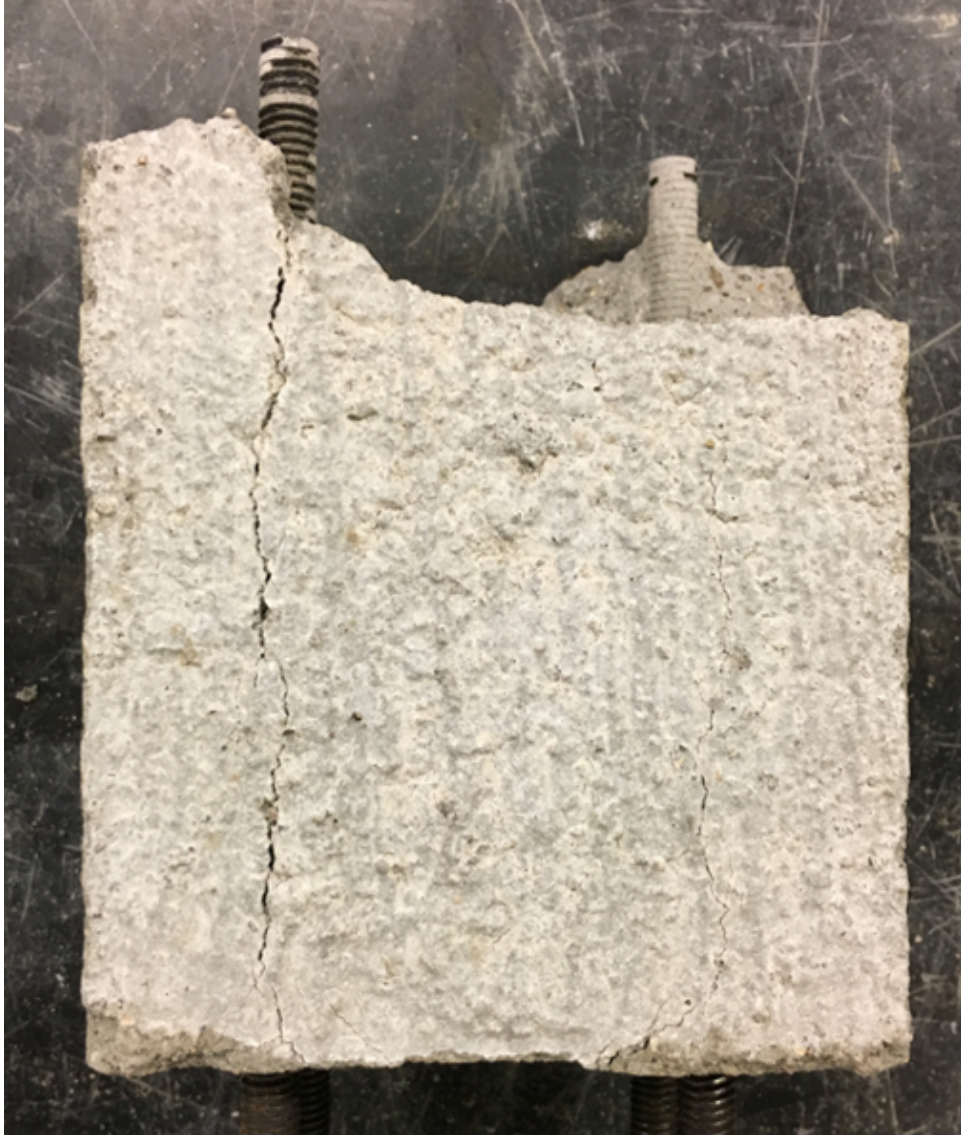
Figure 44 – Specimen #5 surface cracking
