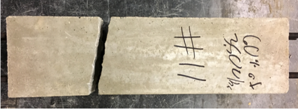
Figure 55 - Specimen #11 failure plan view
