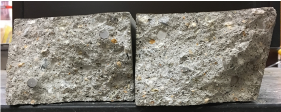
Figure 41 - Specimen #4 failure cross-section
