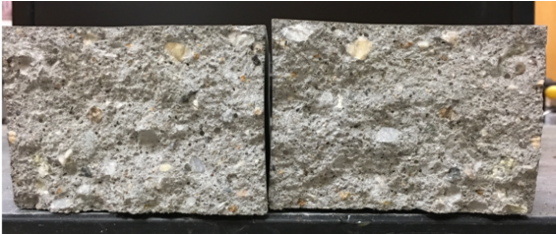
Figure 50 - Specimen #8 failure cross-section
