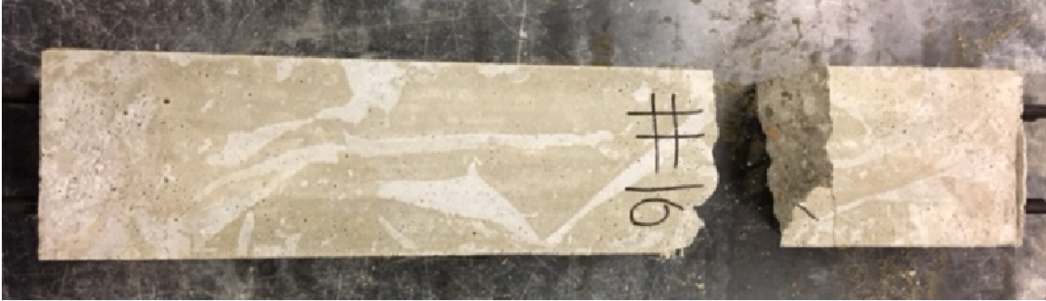
Figure 67 - Specimen #16 failure plan view
