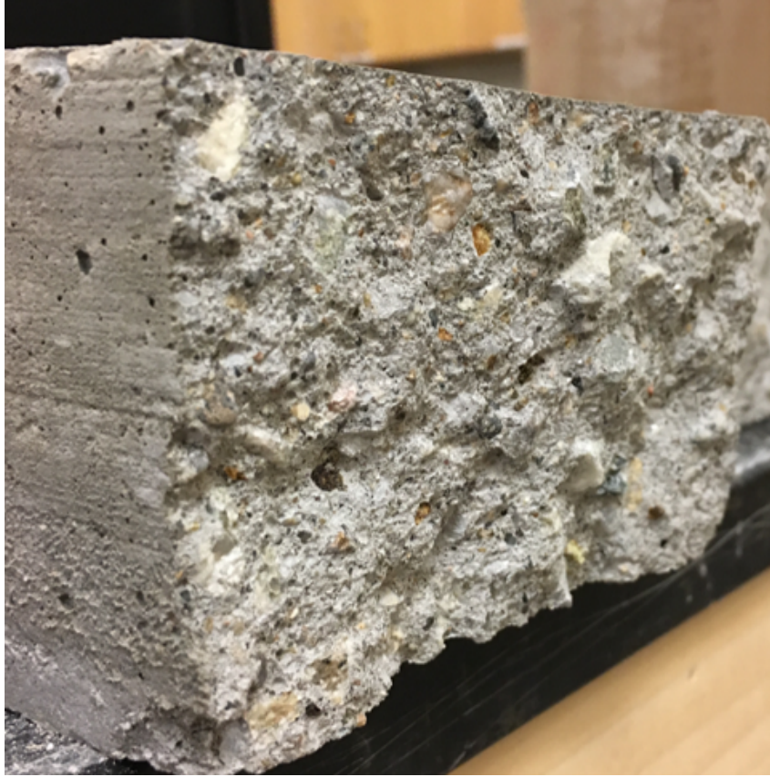
Figure 57 - Specimen #11 failure path
