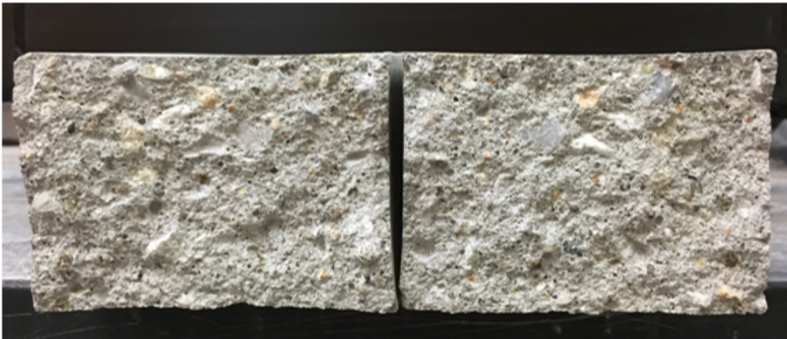
Figure 52 - Specimen #9 failure cross-section
