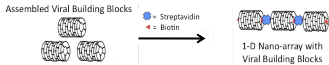
Figure 4.1 Schematic representing the synthesis of a one dimensional nanoarray using doubly biotinylated viral building blocks with streptavidin
