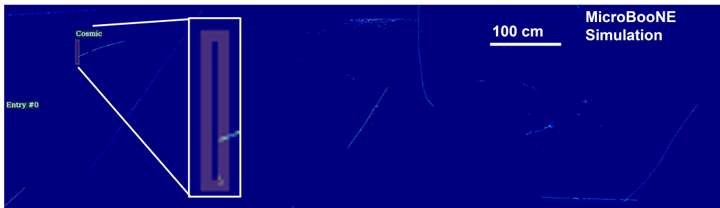
Figure 8.11: A zero-efficiency true interaction almost entirely in a region of unresponsive wires. The white box shows a zoom-in of the area of interest, and within it, the colored box should contain true neutrino interaction. However, because this interaction falls in an unresponsive region of the detector, no deposited charge is seen inside the colored box.
