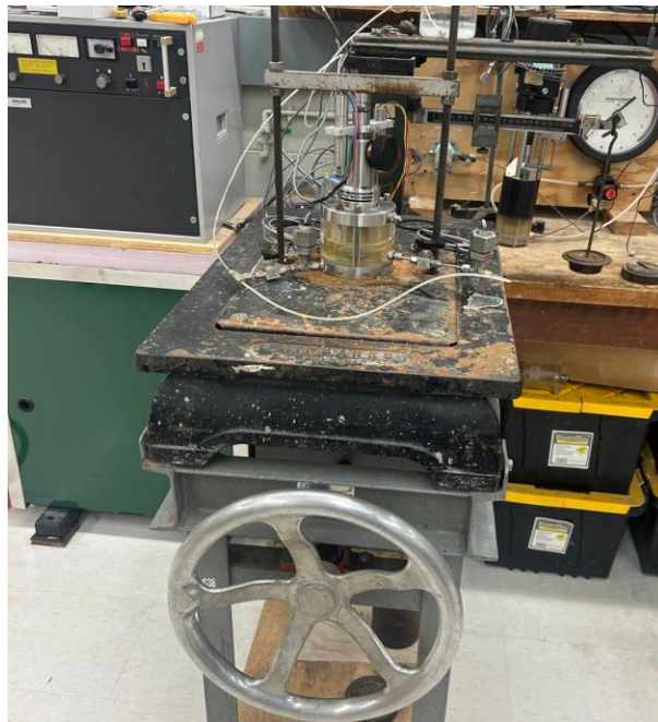
Figure 4-11 MIT Load frame and CRS cell used for oedometer testing
