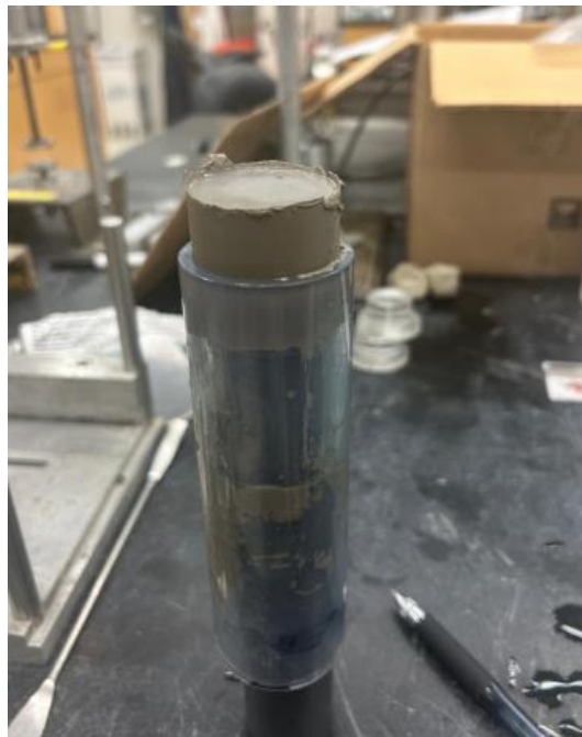
Figure 3-12 CRS sample being extruded from consolidometer before the trimming process.
