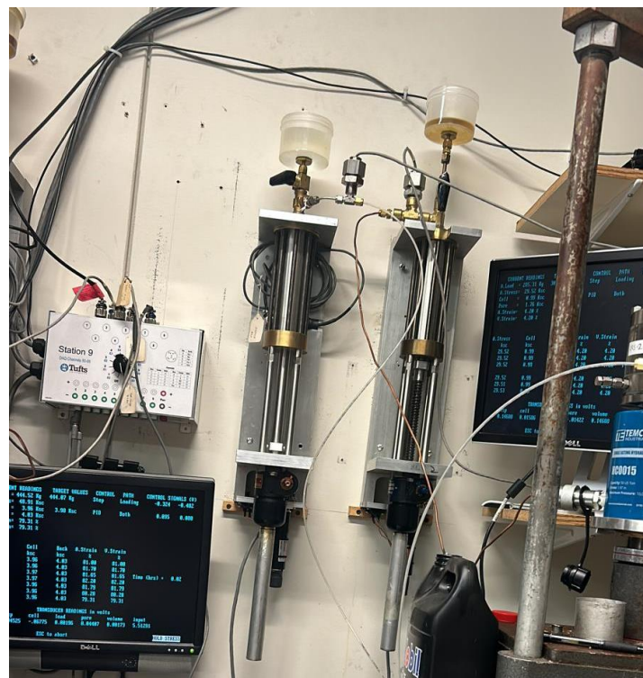
Figure 4-9 Wall mounted PVA's controlling load and cell pressure
