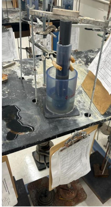
Figure 3-11 Incremental sample loading – Includes consolidometer and axial loading being applied.
