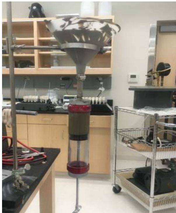
Figure 3-10 Deposition suction gun used to tremie the slurry into the consolidometer.
