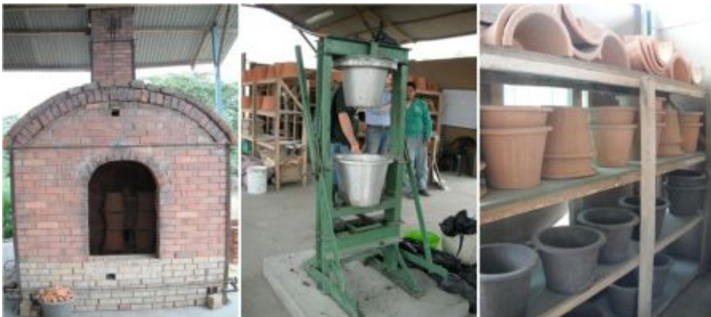
Figure 48: From left to right: the kiln, the press, and tested, fired, and drying filters 2012 [98]
