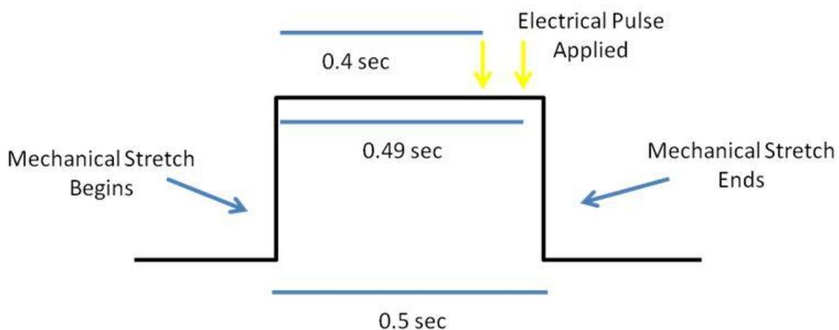
**Figure #6 – A diagram of how electromechanical stimulation was applied. This system allows for electrical stimulation to be triggered by or occur a set amount of time after mechanical stimulation began. That set amount of time is called the delay time.**
