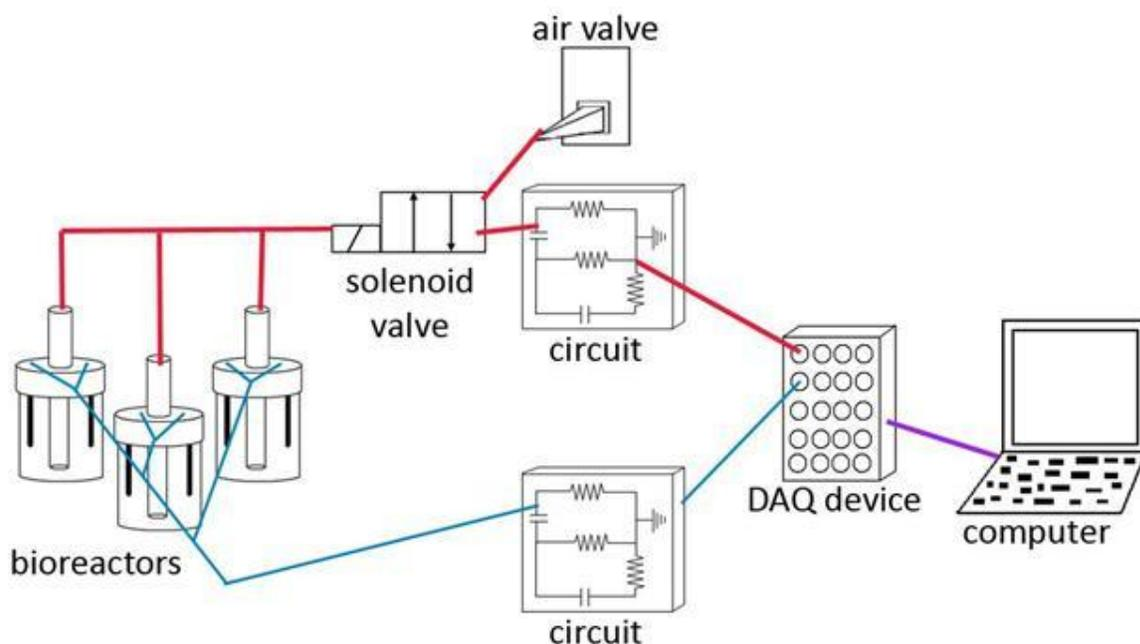
**Figure #5 – A diagram of the system controls and how the individual components interface with each other. The DAQ device and the custom made LabVIEW program are able to control both mechanical and electrical stimulation at the same time through electrical connections.**
