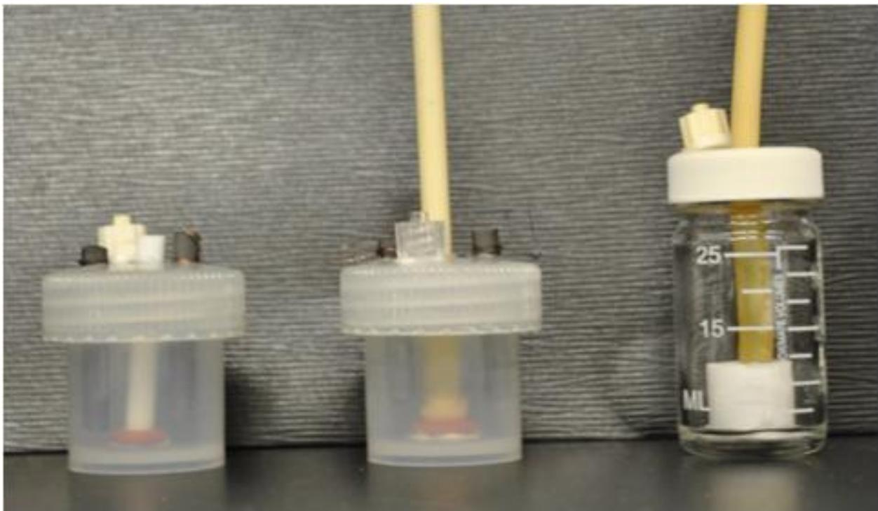
**Figure #4 – A picture of the bioreactors we designed. Pictured from left to right: electrical bioreactor, electromechanical bioreactor, and mechanical bioreactor.**
